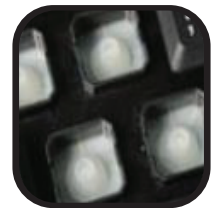
Quiet Membrane Key Switch
